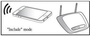
Step 4, Turn on power to the socket after promoted by your network controller inclusion mode. The dt Smart Bulb will be included into your network within 30 seconds. The smart bulb will flash 2 times after Inclusion is successful.
