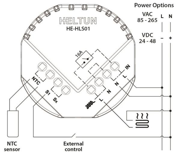
Figure 5: Connection diagram 2
