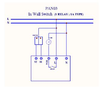
Fig 1. PAN03 Assembling
