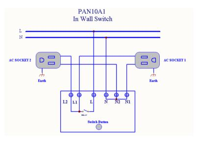
Fig 2. PAN10 Assembling
