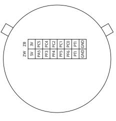
Pins in the ZB row (except for 3V and GND pins) are pins of the Zigbee/Thread/BLE EFR32MG21 chip. Pins in the ZW row (except for 5V and GND pins) are pins of the Z-Wave ZGM130S chip.
